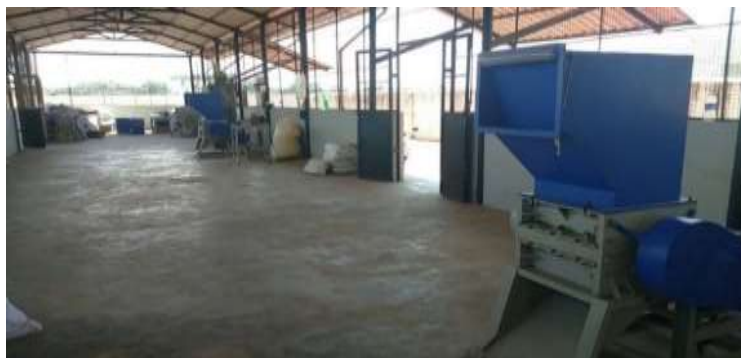
Fig 1. Shredding of PET Waste
