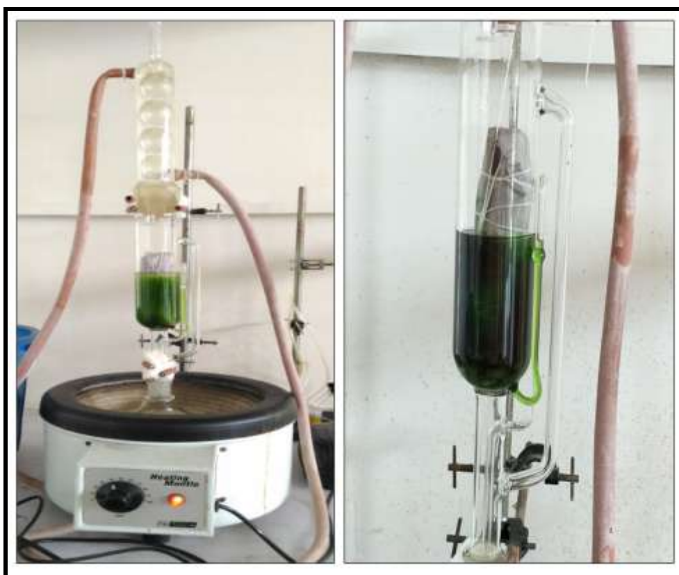
Figure 2 Photographs of Soxhlet Extraction Method Using Different Organic Solvents
