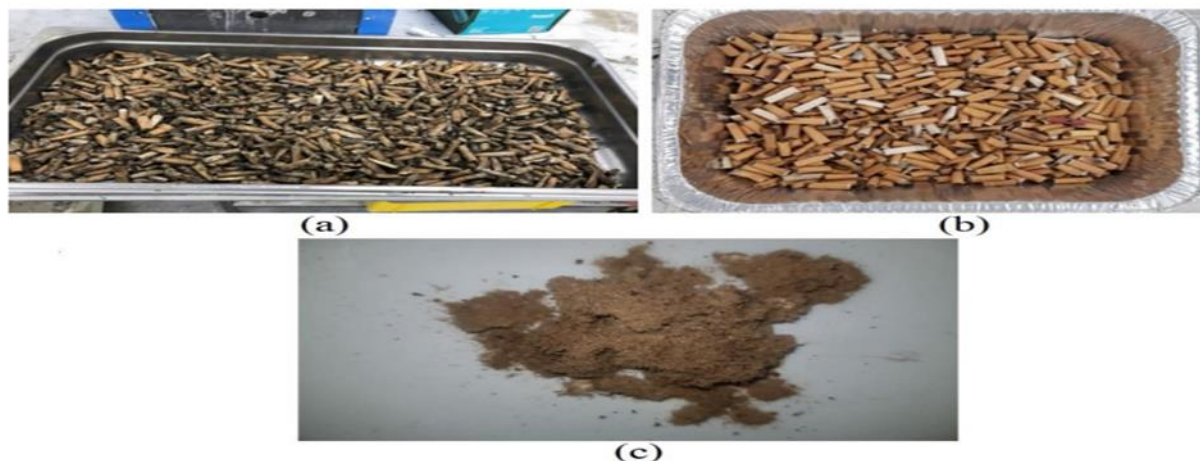
Figure 2: Cigarette butts (a) before to oven drying and (b) after the removal of extra tobacco and debris. (c) Grounded CBs used to prepare samples.
