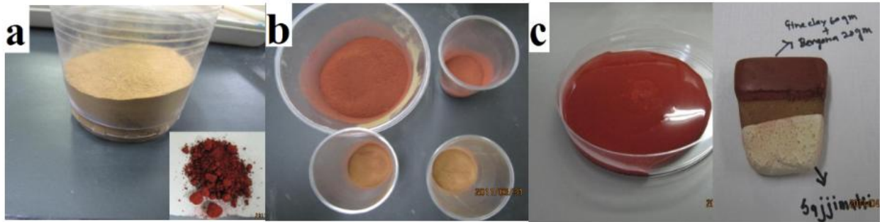
Figure 7: Fine clay and Bengara mixture slip; (a) Fine clay and Bengara powder; (b) Fine clay and Bengara was mixed into different ratio; (c) Prepared slip and applied on the surface of the test piece.
