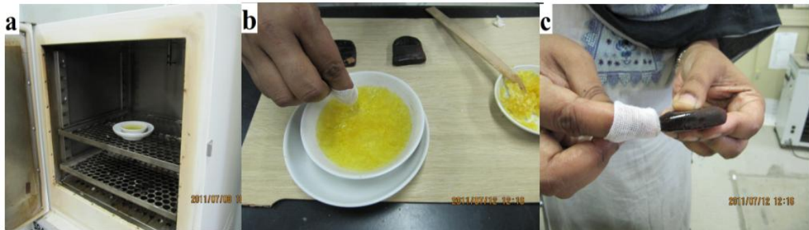
Figure 12: Applying the tung oil as top coating; (a) Tung oil was heating an oven for 24 hours at 120°C; (b) After take out from the oven, oil was applied on the test piece by using a cloth; (c) Applying the Tung oil on the surface of the test piece.
