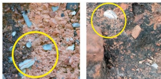
Figure 5: Zoomed in photo displaying particles of snail shells: Ghanasyam Mortar (left), Namath Kali Mortar (Right)
