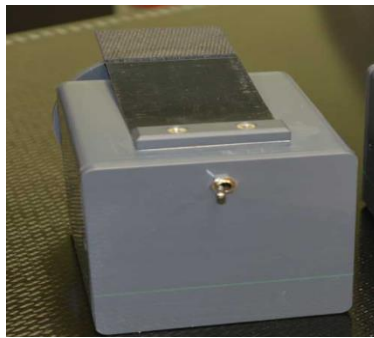
Figure 3: a) Breathing Phantom Figure 3: b) Gating Window displays breathing pattern
