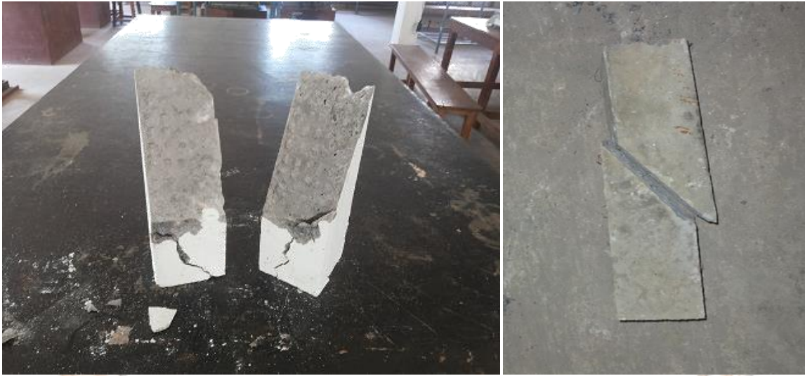
Fig: 4.2.6.4 Failure pattern after testing in 45 degree angle of interface
