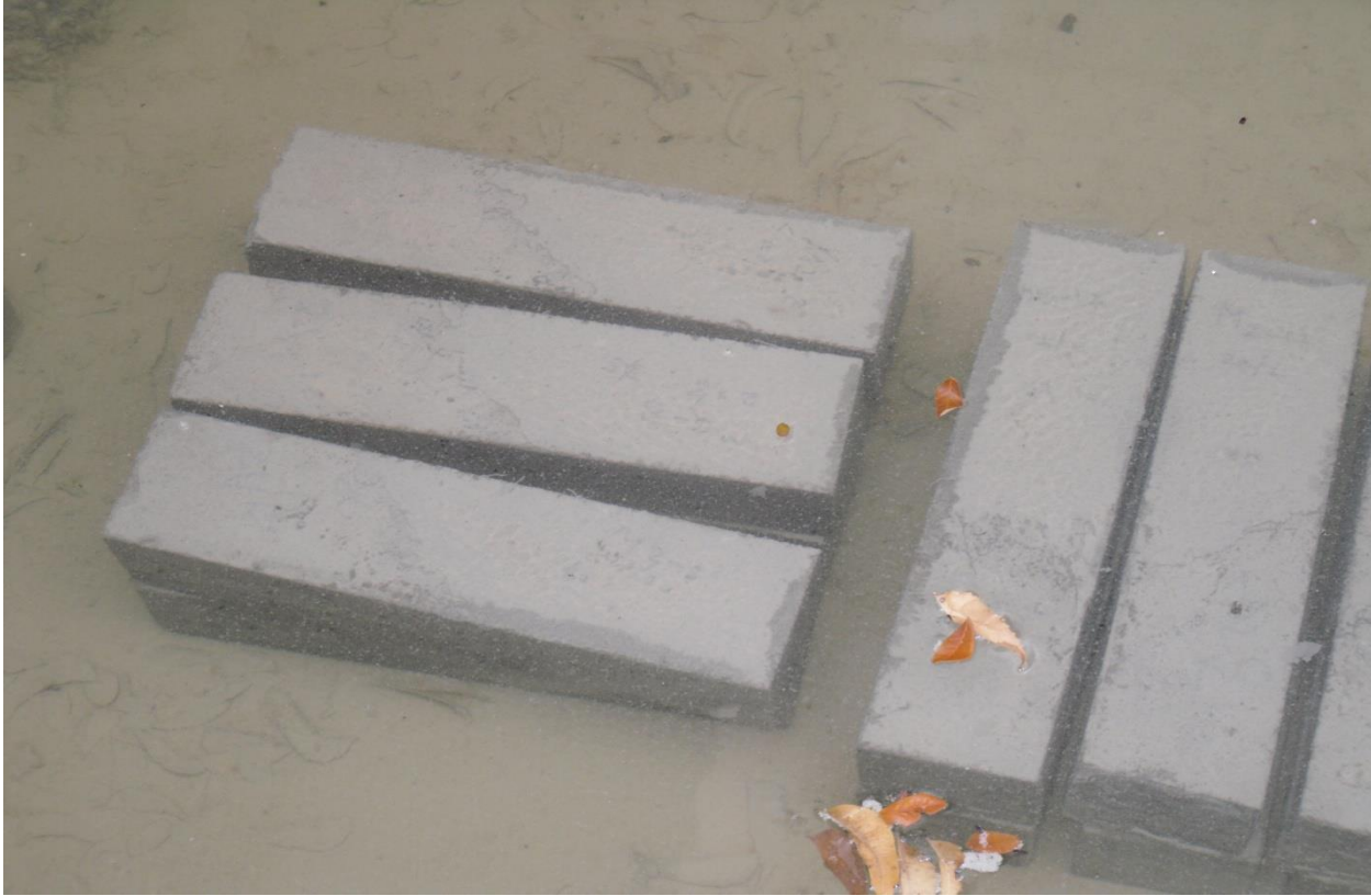
Fig. 3.6.2 Specimen after adding new substrate to the above old substrate kept for curing
