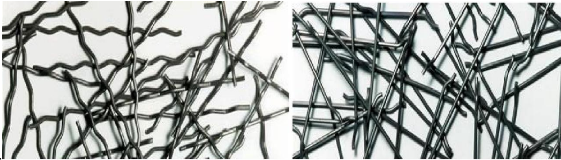
Fig.1.3.2 Typical fiber types used in concrete:
