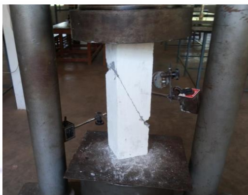
Fig: 4.2.6.1 Initial failure pattern in 30 degree angle of interface
