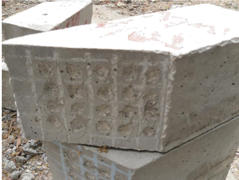
fig: 3.5.2 Specimen that had chipped at regular intervals after 28 days of curing at 45°
