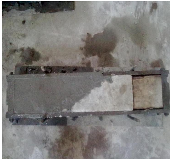
Fig. 3.5.3 Casting of new substrate over the old substrate
