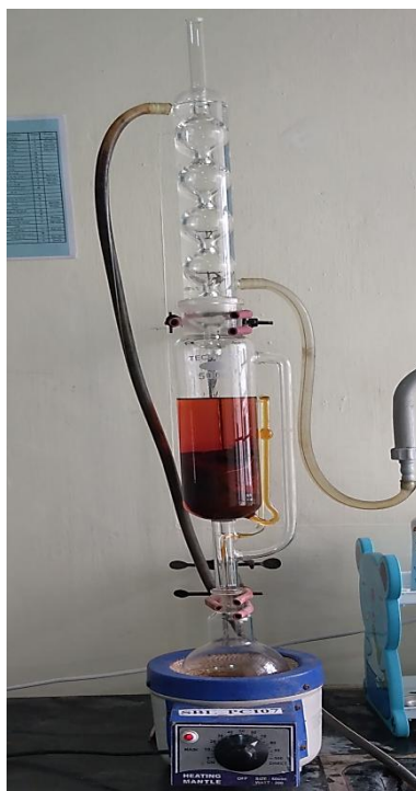
FIG1SOXHLET EXTRACTION OF ALPINIA OFFICINARUM
