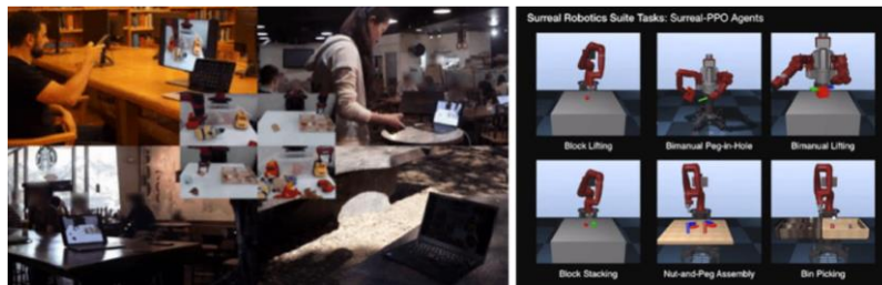
Fig. 2 Roboturk remote learning data collection platform. Source [1]
