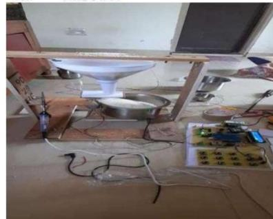
Here we can see the working model which was produced to show the working of the actual model. Here we can see the basic components like arduino uno, servo motor, RFID reader, LCD display and keypad. Here when we put the authentication code and tap the card it showed the correct detail on the led display and then it dispenses the right amount of ration. After dispensing the ration, it also shows "thank you" message also.
