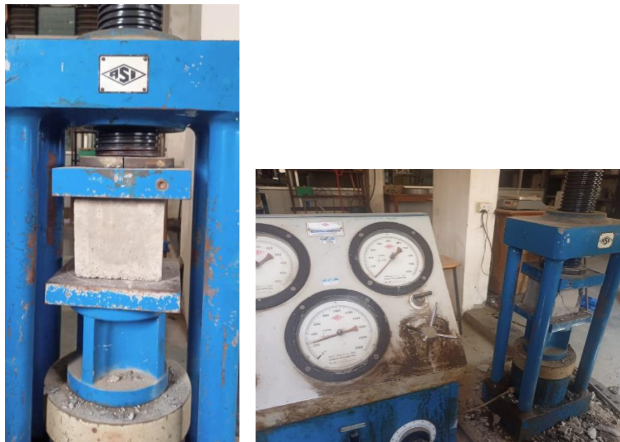
Figure 7 Transparent concrete block in UTM.
