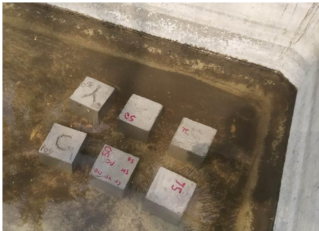
Figure 5 Curing of block
