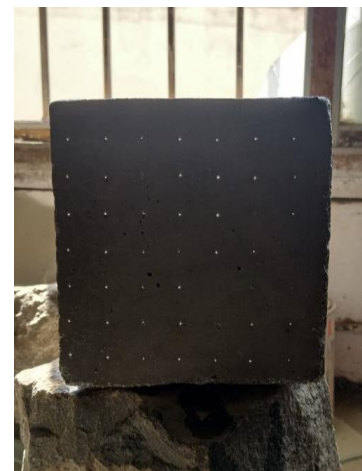
Figure 6 Transparent concrete block
