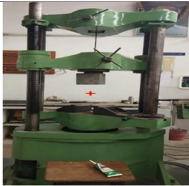
Fig 4. Experimental setup for finding the bond strength
