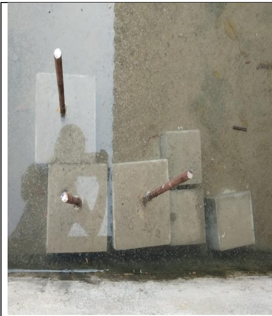
Fig 3. Cubes with 12mm diameter steel bar with the embedded length is 90mm
