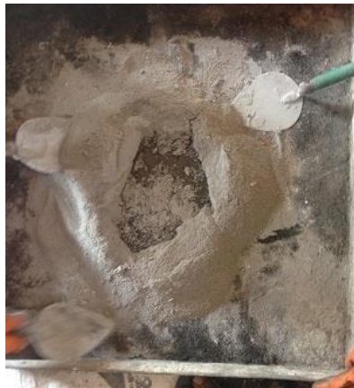
Adding alkaline solution to dry mix
