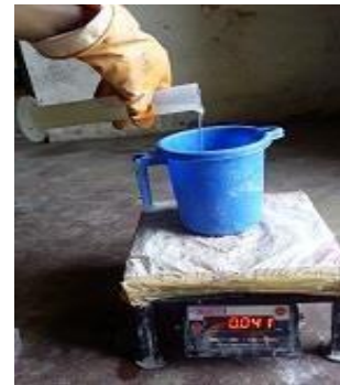
Mixing of NaOH solution with \text{Na}_2\text{SiO}_3
