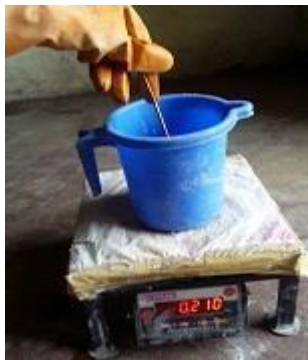
Dissolving of NaOH with water
