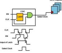
This is a simple illustration of clock gating . The clock signal to the registers is gated with a control signal that selects which functional unit is in use .
