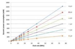
Above chart illustrates how selecting different clock frequencies impacts the dynamic power profile. You can also see how dynamic power consumption increases linearly with clock frequency.
