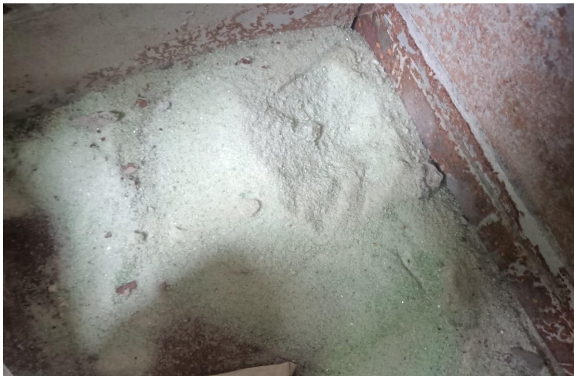
Fig 4: Shows waste glass after sieving and cleaning
