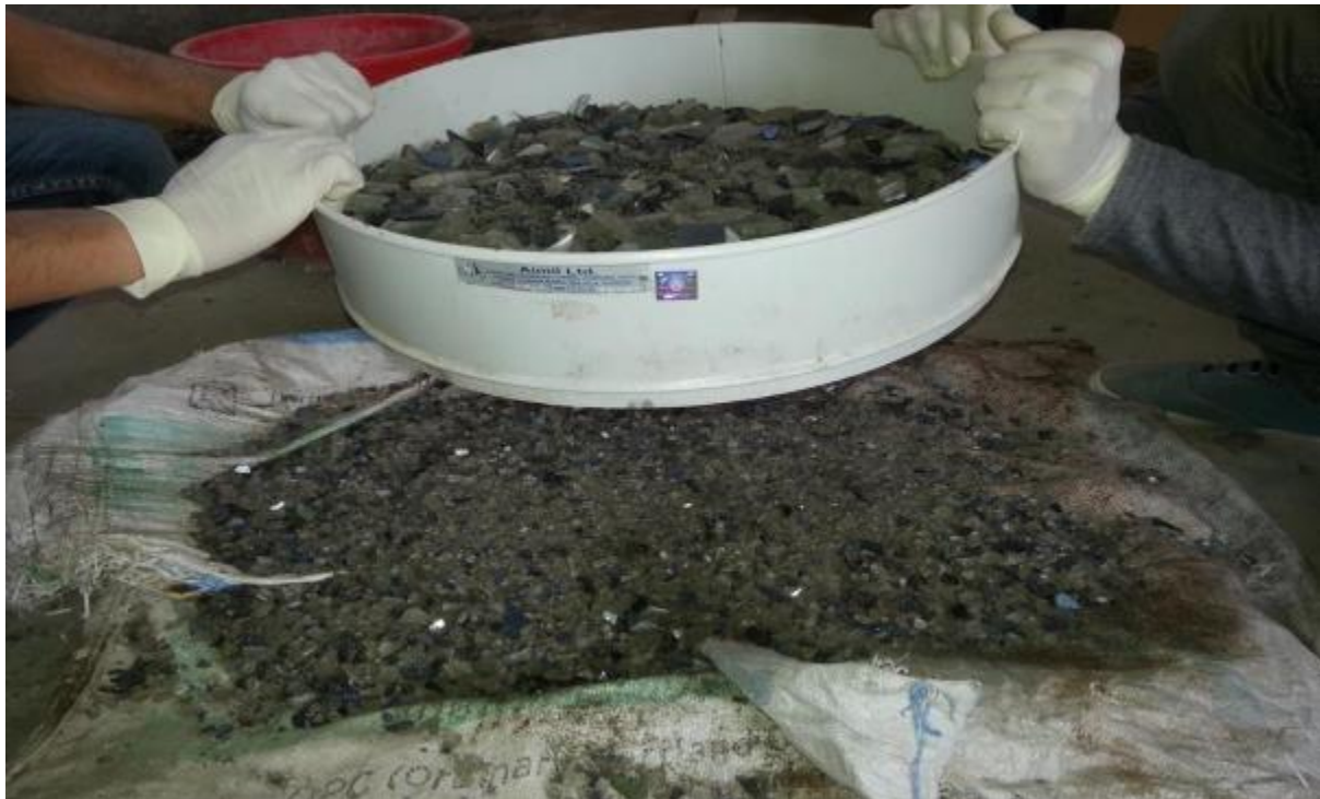
Fig 3 : Shows sieving of waste glass after crushing
