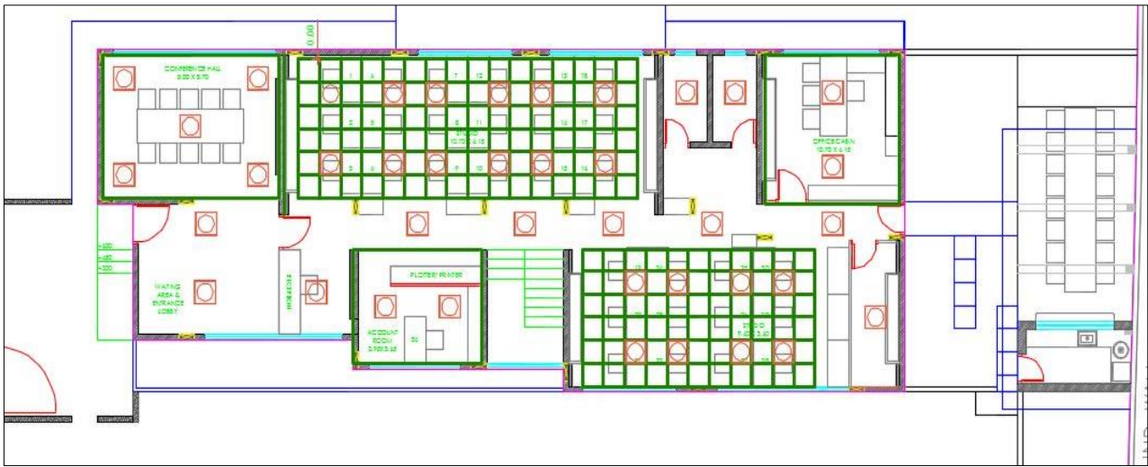
Figure 14: Electrical layout for office floor
