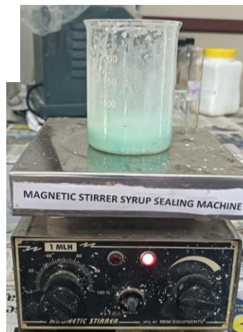
Figure 5 : Preparation Of Casting Solution In Magnetic Stirrer
