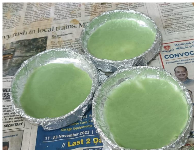
Figure 6 : Casting Solution Is Poured In A Petridish Containing Aluminium Foil
