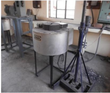
Electrical Resistance Furnace
