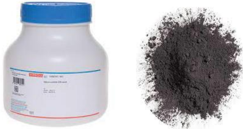
Fig.2 Reinforcement Material: SiC
