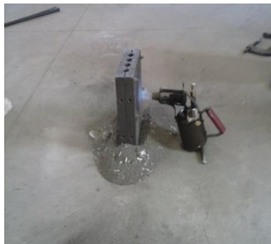
Pre heating the mould box
