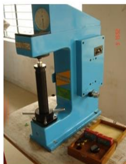
Fig.8 Brinell Hardness Testing Machine
