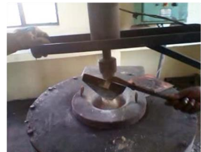
Setting of Stirrer and adding reinforcement
