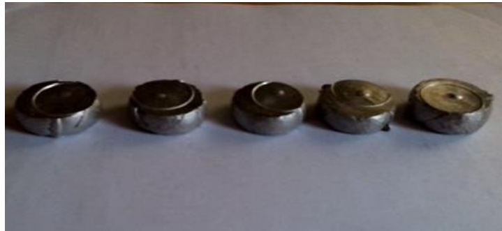
Fig.7 Specimens before and after Compression test
