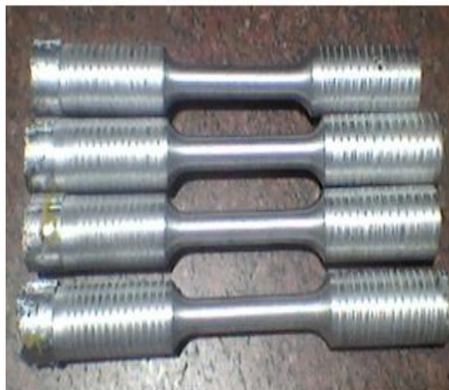
Fig.6 Specimens for Tensile test
