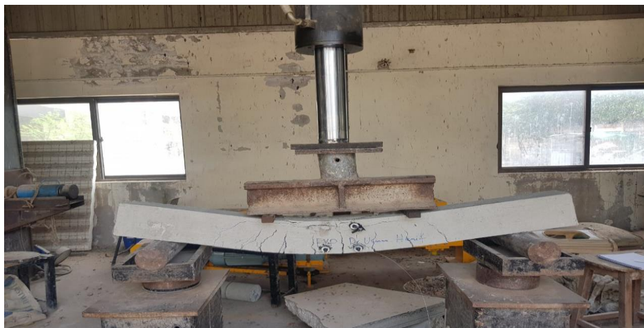
Figure 8: Cracking Induced in Beam due to Loading
