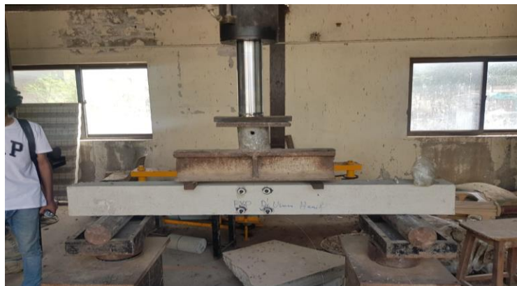
Figure 6: Beam Placed on Loading Rig to Induce Damage
