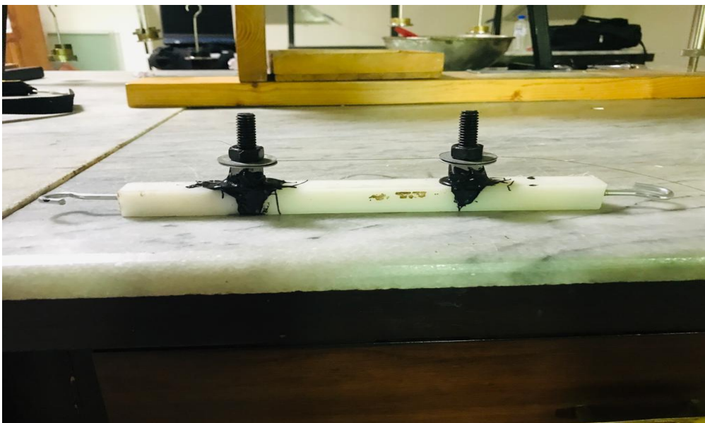
Figure 4: Calibration Gauge Setup on Nylon Bar
