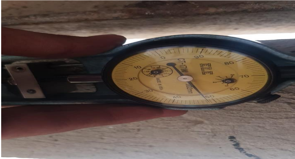
Figure 7: Strain Measurements Using Demec Gauge
