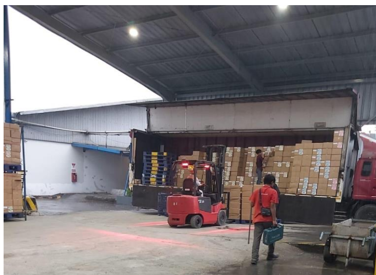
Figure 2. Forklift condition after adding additional lights & buzzer sound
