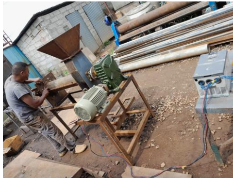
Fig A.4: Assembling work on dewatering machine
