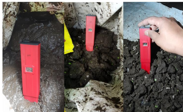
Fig A.5: pH mesurement for the sample before and after sundrying
