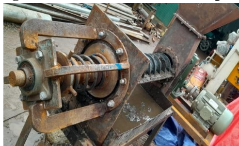
Fig A.2: Complete fabricated system with pressure cone
