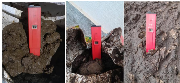
Fig A.6: pH mesurement for the pretreatment of sample before dewatering
