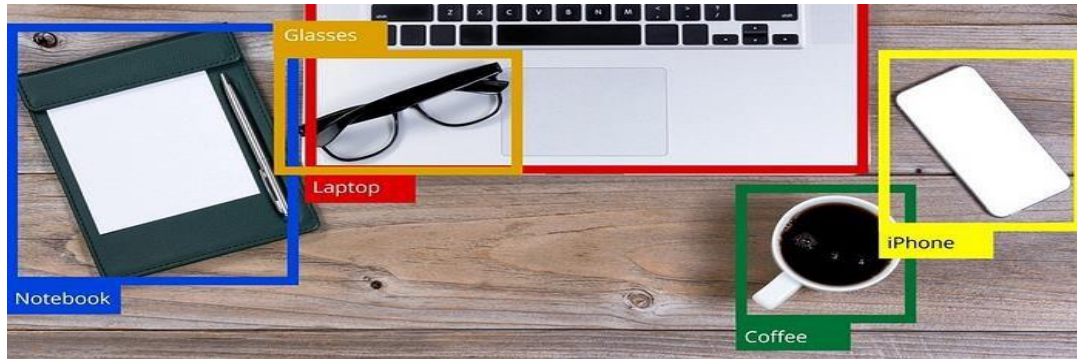
Fig 8: Output from SSD MobileNet Object Detection Model
