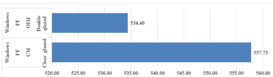
Fig. 17. Impact of Window Insulation (First Floor) on SAIV - CM vs. OIM(KWh/m 2 )
