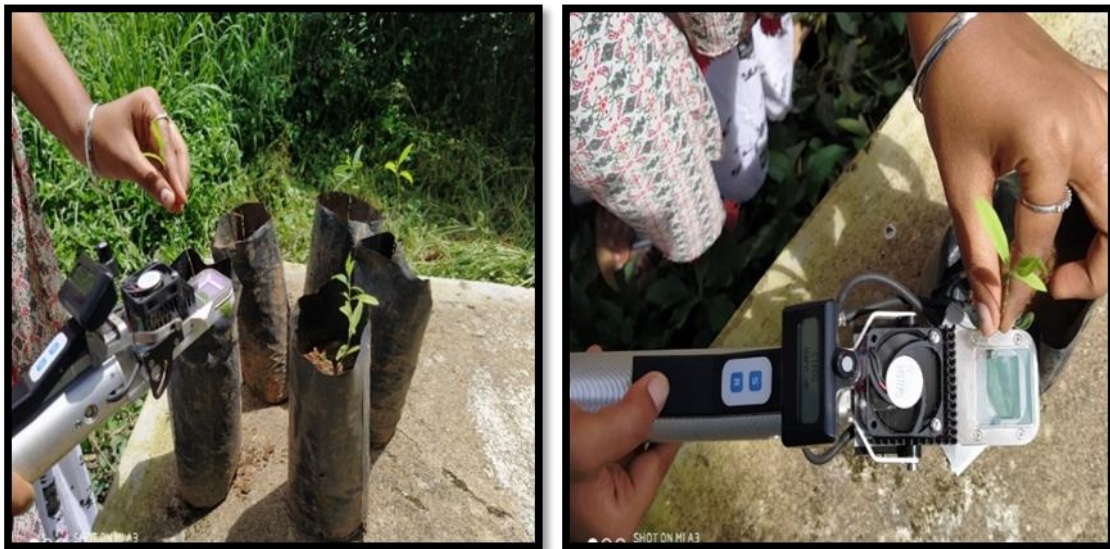
Fig A.1: Physiological parameters measurements using Portable Photosynthesis System Meter (PPS Meter)
