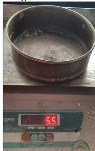
Fig.4.6 Retained residue of the cement sample weighed
