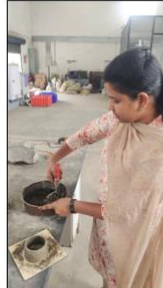
Fig.4.3 Mixing of cement and water
