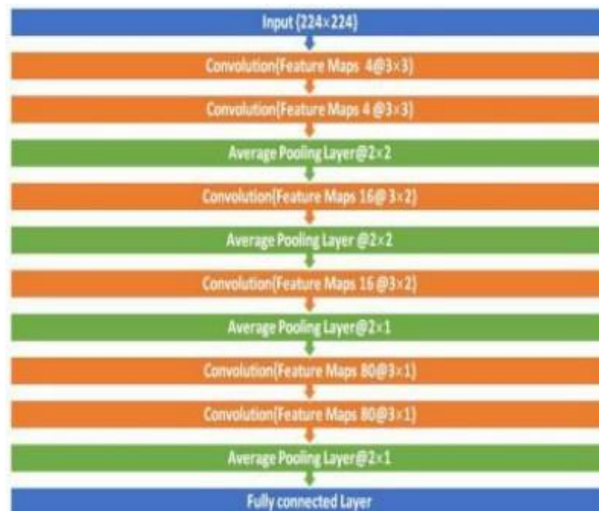
Fig. 8. Archetecture of CNN of perposed System
