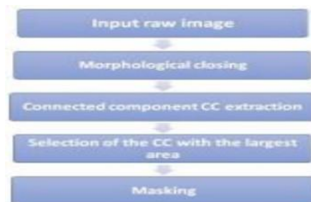
Fig. 10. Segmentation steps for pre-processing.
