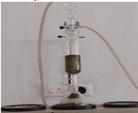
Figure No :8 Soxhlet Extraction process
