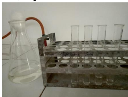
Figure No :14 ( Dilution of Phenol Stock solution 1:1000 1:1200, 1:1400, 1:1600)
