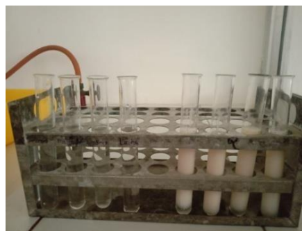
Figure No :15 ( Dilution of Test Disinfectant, Dettol solution 1:100, 1:120, 1:140, 1:160)
