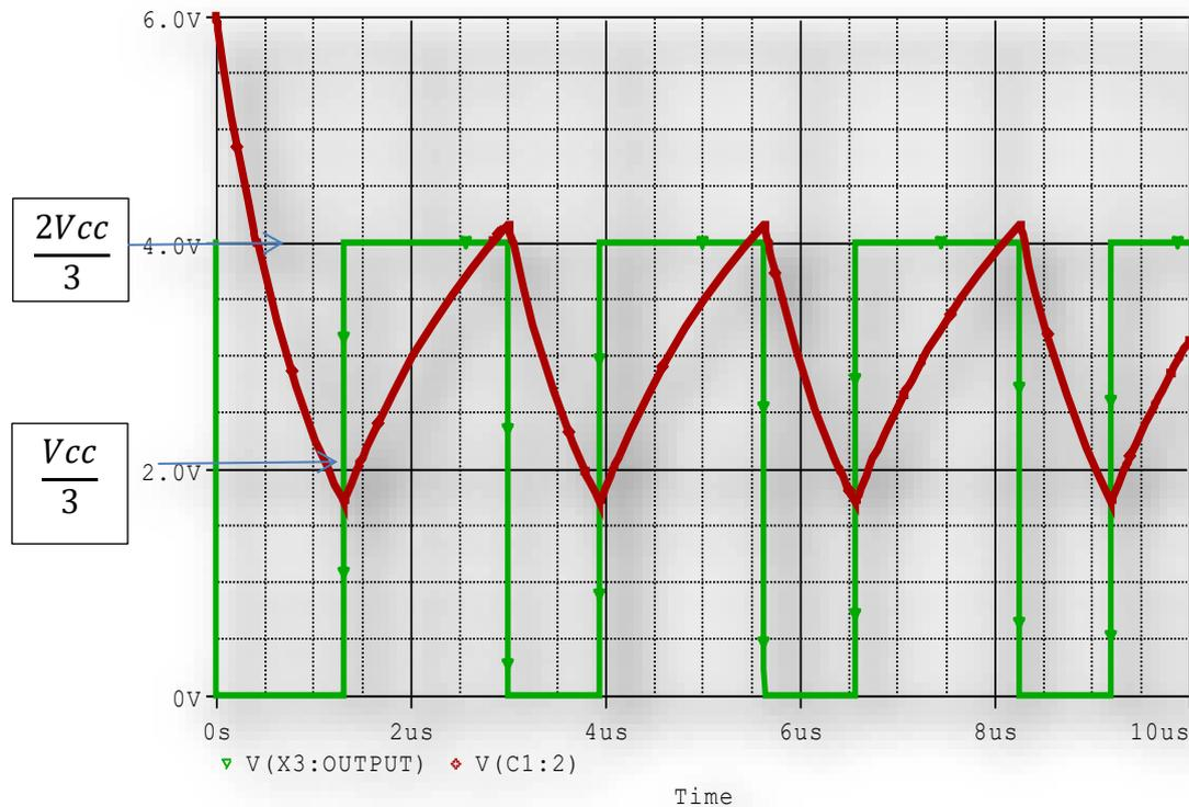
**Figure: 9 The capacitive and output voltage from the sensor**
