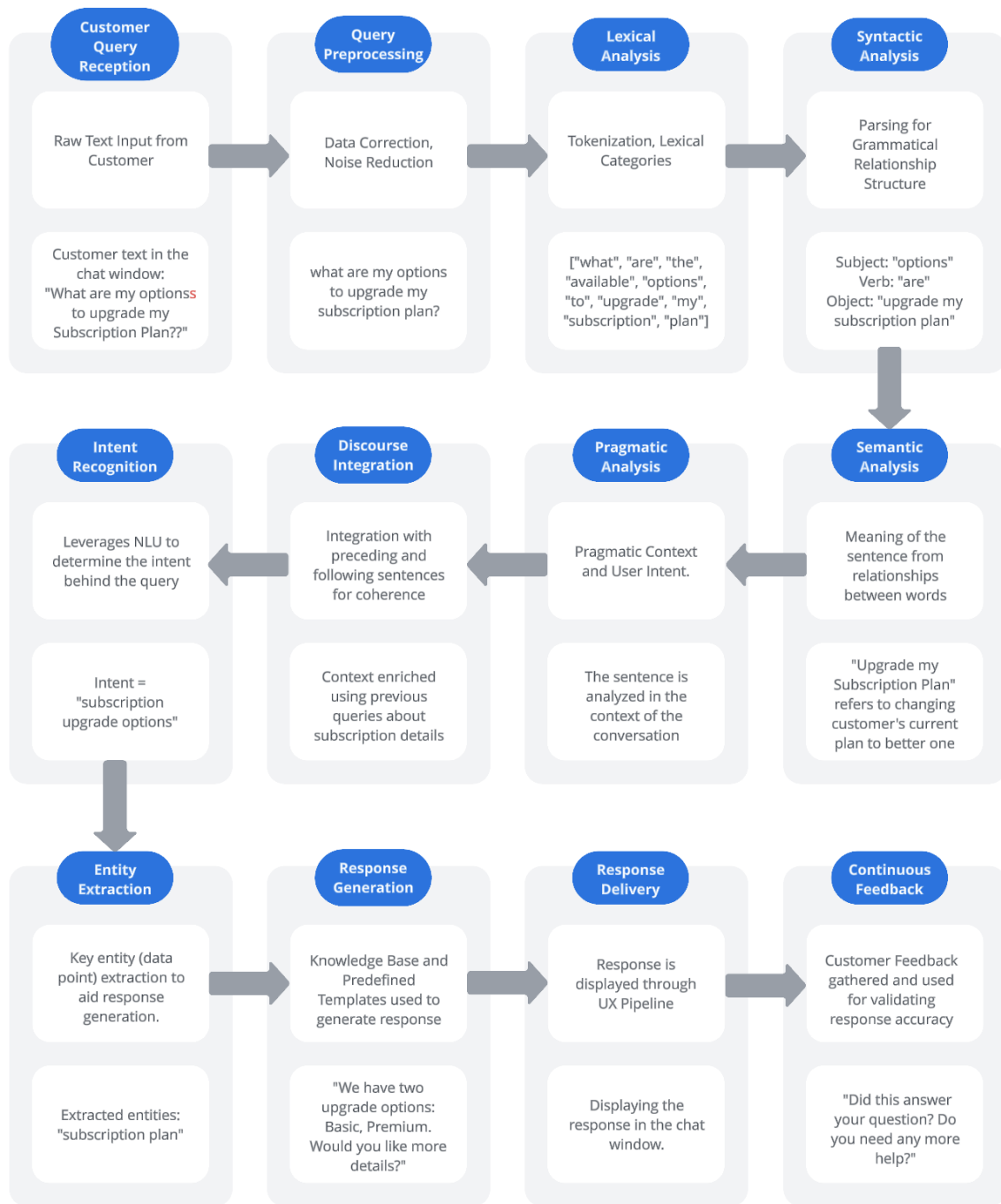
Figure 2. Workflow of NLP and NLU in processing a chatbot customer query
