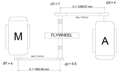
Diameter of first pulley D1=4 inch Diameter of second pulley D2=5.5 inchDiameter of third pulley D3=7 inch Diameter of fourth pulley D4=5 inch Motor speed=1500
