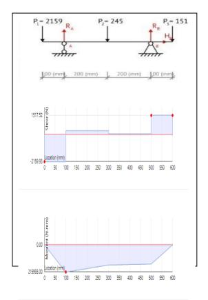
Reaction forces at both bearings RB+RD =2159.93+245+1517.52 =3922.45 Moments about B -(100\*2159.92)+(200\*245)-(RD\*400)+(1517.52\*500)RD\*400 = 591767 =591767/400 RB=1479.41 N Moment about D
