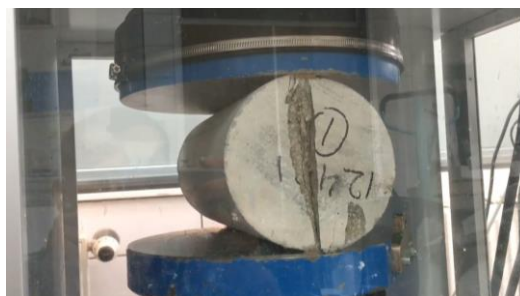
Fig. 2: Splitting tensile test of cylinder
