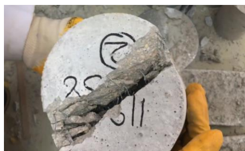
Fig.3: cylinder in two halves at failure
