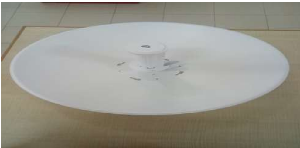
Figure 3: Rocket Dish-5G30 Antenna
