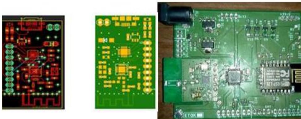
Figure 4: Node PCB Design & Gateway Circuitry
