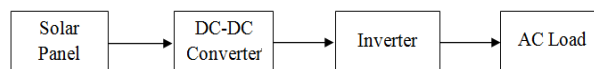
Fig 1.The basic block diagram of the solar energy conversion system for ac load
