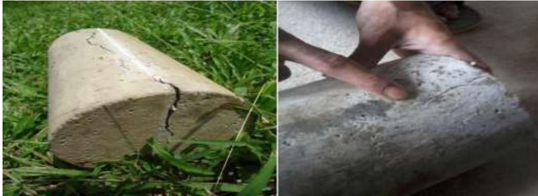
Figure 1.17: Cracking pattern of Conventional concrete and coconut fibre reinforced concrete
