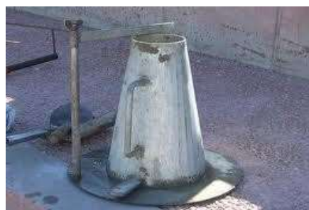
Slump Testing Apparatus Fig 1.4
