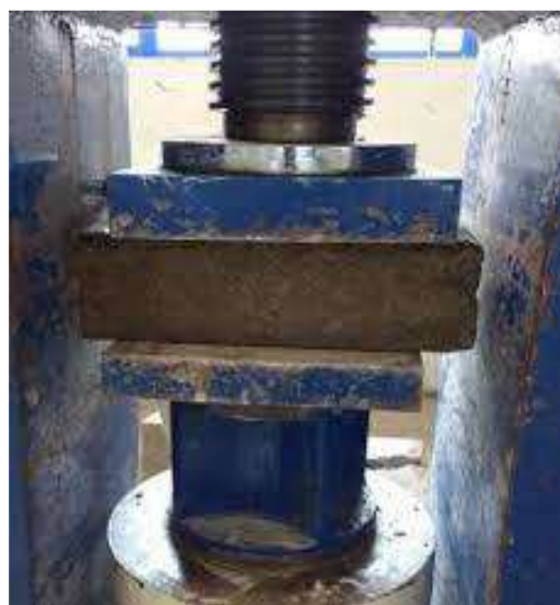
Figure 6: Finding the compressive strength of brick using compressive testing machine
