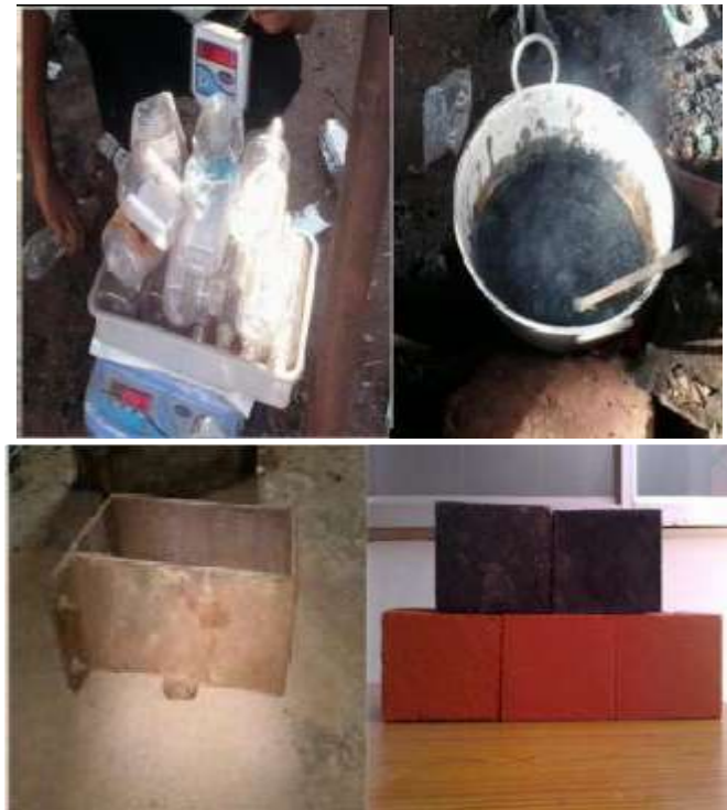
Figure-5: preparation of plastic brick specimen
