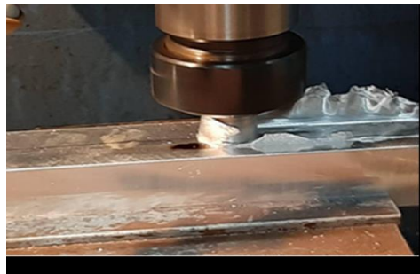
Figure 3. Friction Stir Welding (FSW) Process on AA 6063
