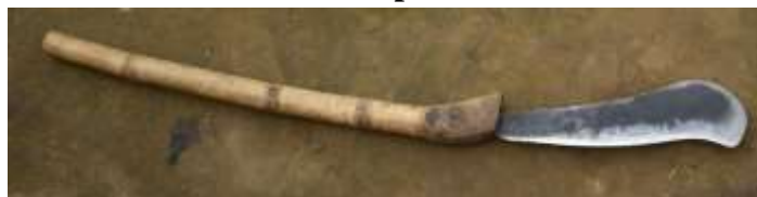
Image 5: Khangra (variety 3) with less depth at the working edge and broader width at the curve-point
