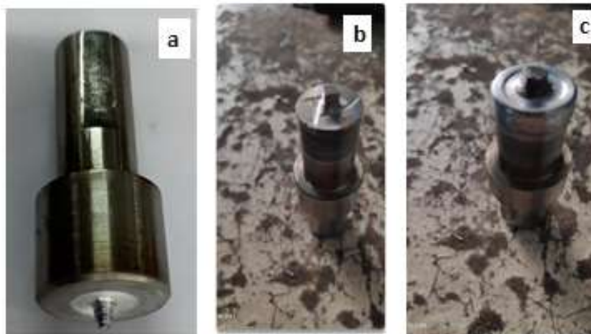
Figure 1. FSW Tool Profiles (a) Tapered Threaded [TTH], (b) Square Cylindrical [SQC] and (c) Hexagonal [HEX] configurations.
