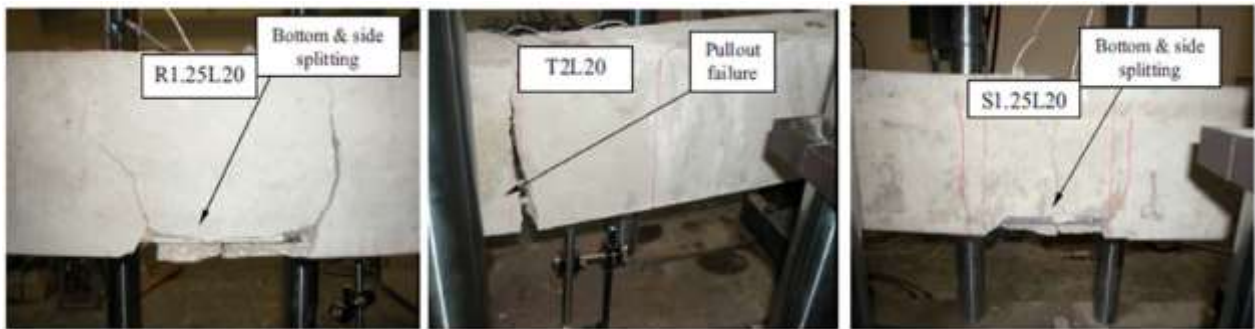
Fig. 12 Bond failure modes of beam specimens
