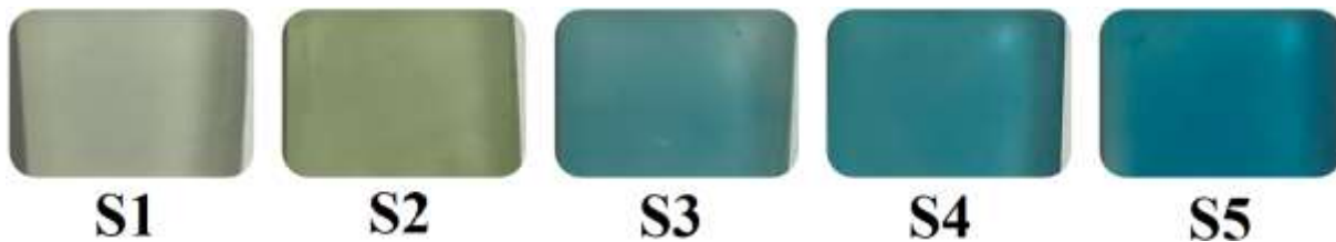
Fig. 2. Photographs of optically polished glass samples prepared for optical characterization.
