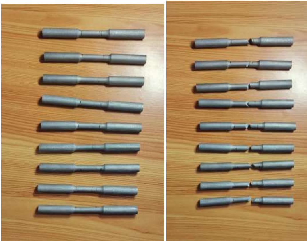
Figure 5: UTM L9 samples and after experimental braked samples.
