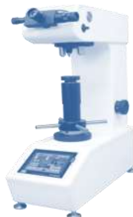
Figure 7: Vicker hardness tester.
