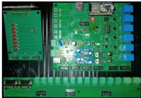
Figure 3. Final PCB prototype of the HMI board.
