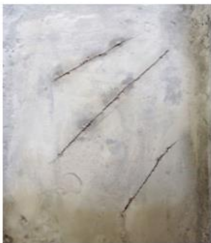
Fig no.6. Concrete before inoculation of culture (crack size- 2 mm)
