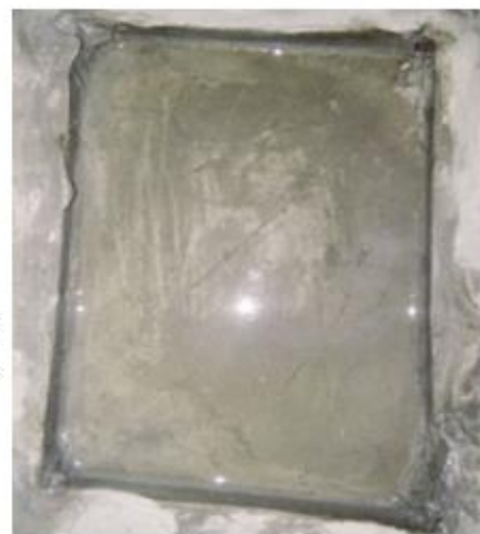
Fig no.7. Concrete after inoculation of culture (crack size- 1 mm)
