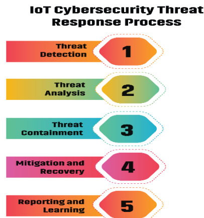
Figure 4: Flow chart illustrating the IoT cybersecurity threat response process.
