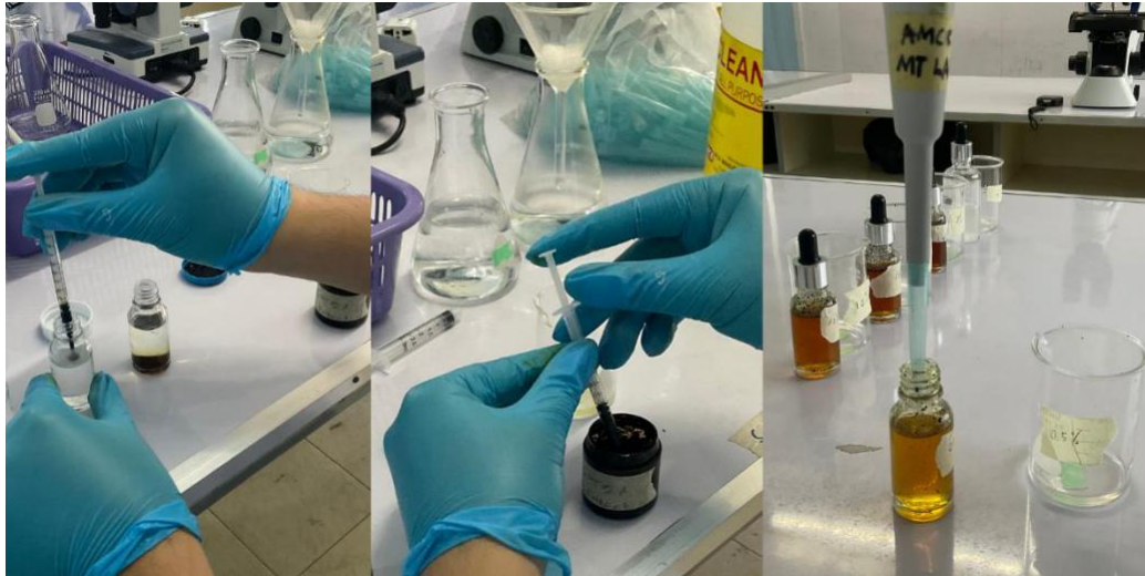
Figure 6. Dilution of Hibiscus rosa-sinensis leaf crude extracts into four different concentrations (0.5%, 1.0%, 1.5%, and 2.0%)
