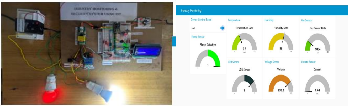
“Figure 4. System Is In ON Condition”
