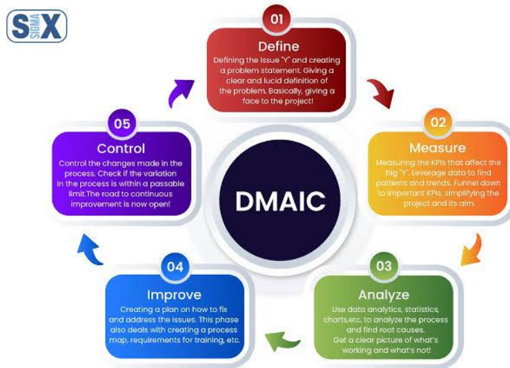
Fig.2: Flowchart of DMAIC Process in Lean Six Sigma
