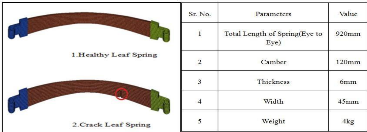
Fig-1: Dimension of leaf spring
