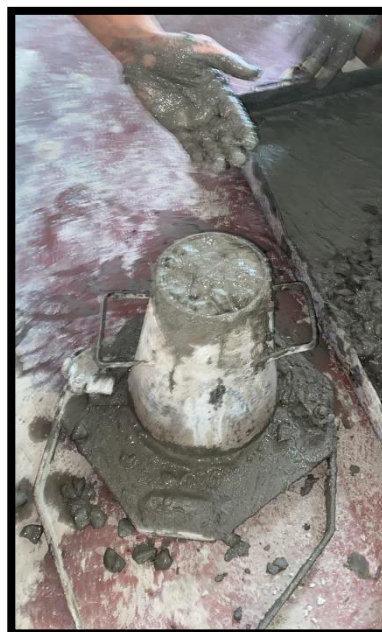
Fig 6. Slump cone test
